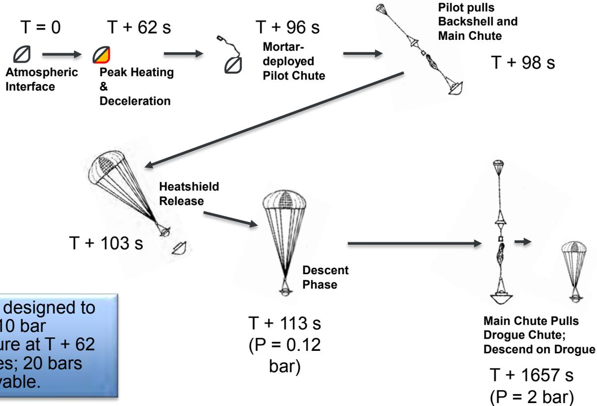
Probe designed to meet 10 bar pressure at T + 62 minutes; 20 bars achievable.
